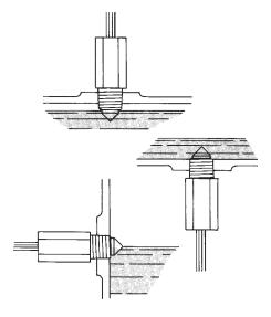
$\underline{\mbox{Note:}}$  Units must be mounted vertically or horizontally.
