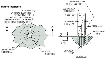
\* If the total area of overseat port is less than the orifice diameter, then the overseat is the restrictor.
