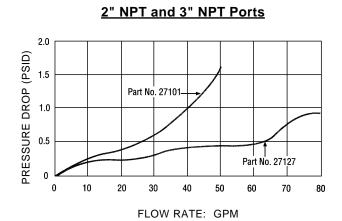
**Note**: Tests conducted with units in horizontal position (lead wires up) with water at +70°F (21°C).
