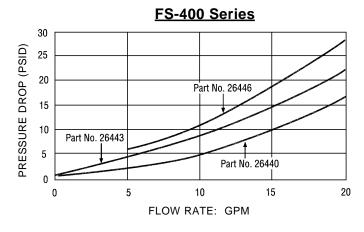
**Note**: Tests conducted with units in vertical position (lead wires up) with water at +70°F (21°C).
