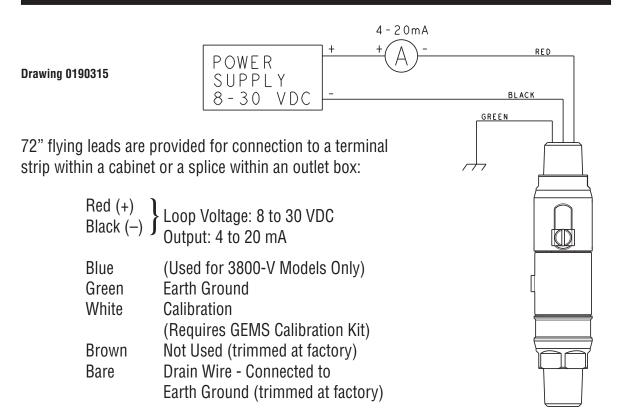
NOTE: An external ground screw is included for additional earth ground connection.
