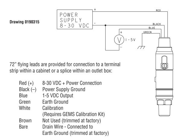
NOTE: An external ground screw is included for additional earth ground connection.
