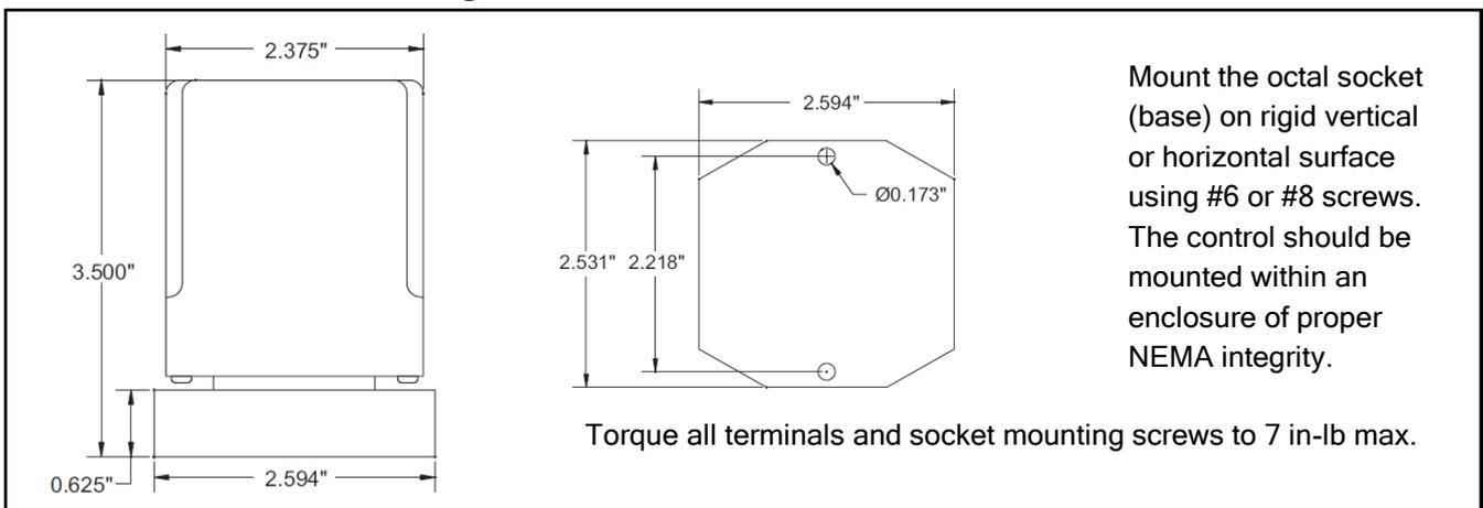
Mount the octal socket (base) on rigid vertical or horizontal surface using #6 or #8 screws. The control should be mounted within an enclosure of proper NEMA integrity.
