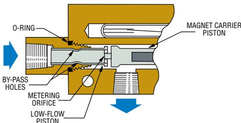
An additional, lap-fitted piston is used in Gems FS-926 Series to accurately detect low-flow rates. Calibration is determined by one or more metering holes in the end of the low-flow piston, which regulate bypass flow, and therefore the actuation setting.
