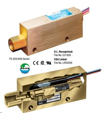
Both the FS-925 and FS-926 use a spring-loaded piston to detect positive flow with great precision. They act upon direct fluid flow and will not show "false-positive" flow indication as can happen with sensors using indirect sensing methods such as pressure measurement. The FS-926 incorporates an additional lap-fitted piston for very low flows; see below.
