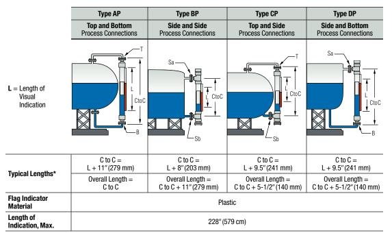
\* Dimensional data varies due to connections, material and specific gravity.
