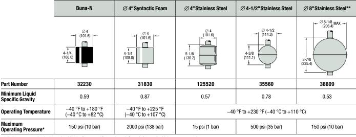
\* Unit pressure rating is determined by the flange and float selected. Consult factory for higher pressure ratings.
