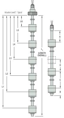
\* Actuation level distances and L<sub>o</sub> (overall unit length)
