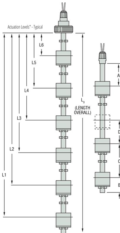
\* Actuation level distances and L<sub>0</sub> (overall unit length) are measured from inner surfaces of mounting plug or flange.
