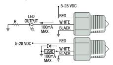
Note: Inductive loads must be diode suppressed.
