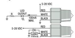
Note: Inductive loads must be diode suppressed.
