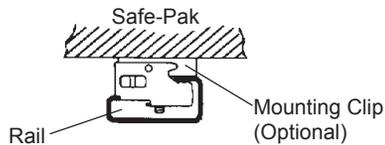
**FIG. 3 Details of Safe-Pak Grounding**
