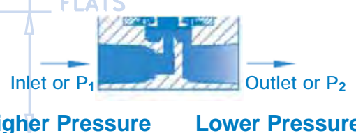
(Figure 1) Pressure differential is the difference between the inlet and outlet pressures.
